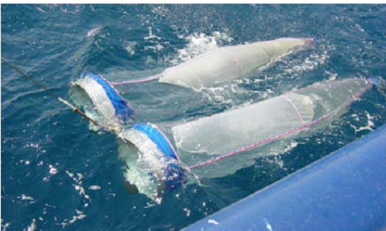
Figure 7. A neuston net (left) was used to sample surface waters and paired bongo nets (right) were used to sample through the water column from surface to near bottom. (photos courtesy Project Oceanica/Leslie Sautter)
