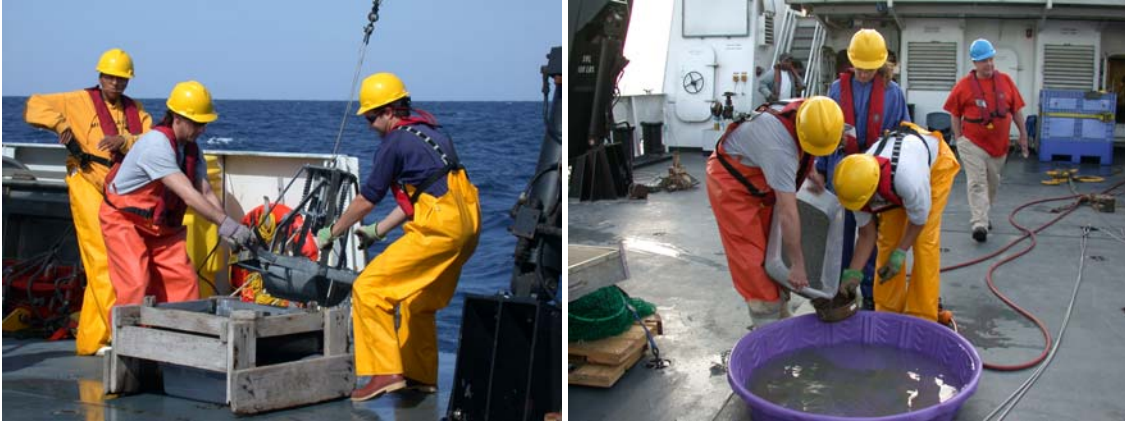
Figure 5. Bringing the Smith-McIntyre grab on board (a) and washing down sediment sample collected by the grab (b).
