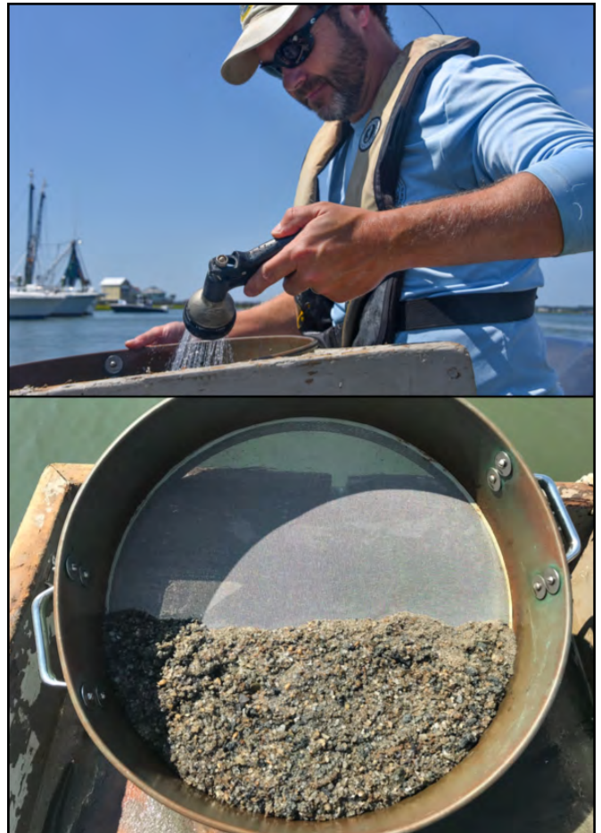
A macrobenthic invertebrate sample is collected and rinsed through a 0.5 mm sieve before being preserved for processing in lab.
