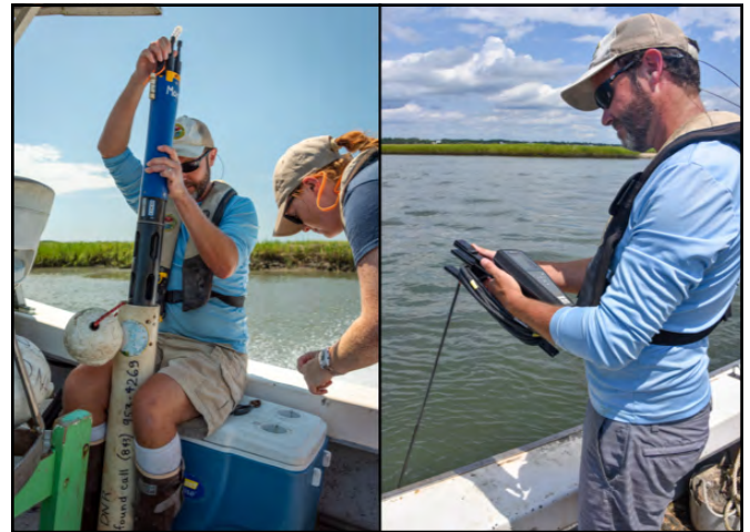
A handheld multi-meter (right) is used to collect water quality at different depths, and a data logging instrument (left) is deployed to collect bottom water quality throughout two high-low tidal cycles.
