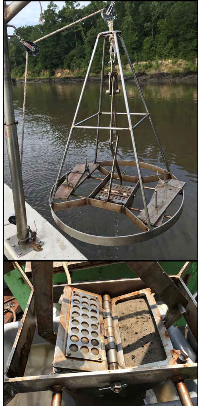
A Young grab is used to collect samples for sediment quality and benthic biological condition.
