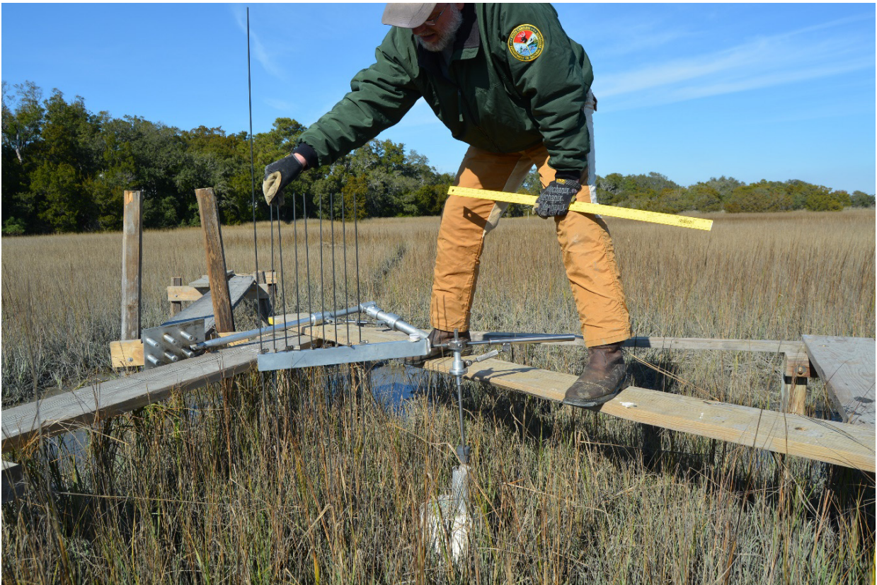
Appendix F, Figure 5. RSET installed with RSET pins being lowered to the marsh platform surface.
