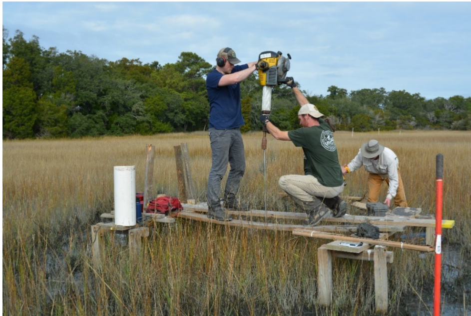
Appendix D, Figure 8. A power hammer is used along with a rod driver attachment (anvil) that screws into the top of the rod being driven (to protect the integrity of the rod, allowing for multiple 4' sections to be screwed together).
