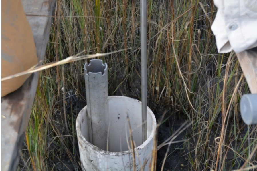
Appendix D, Figure 9. The PVC collar is installed in the center of the measuring plot, enclosing both the rod and the SET insert pipe.
