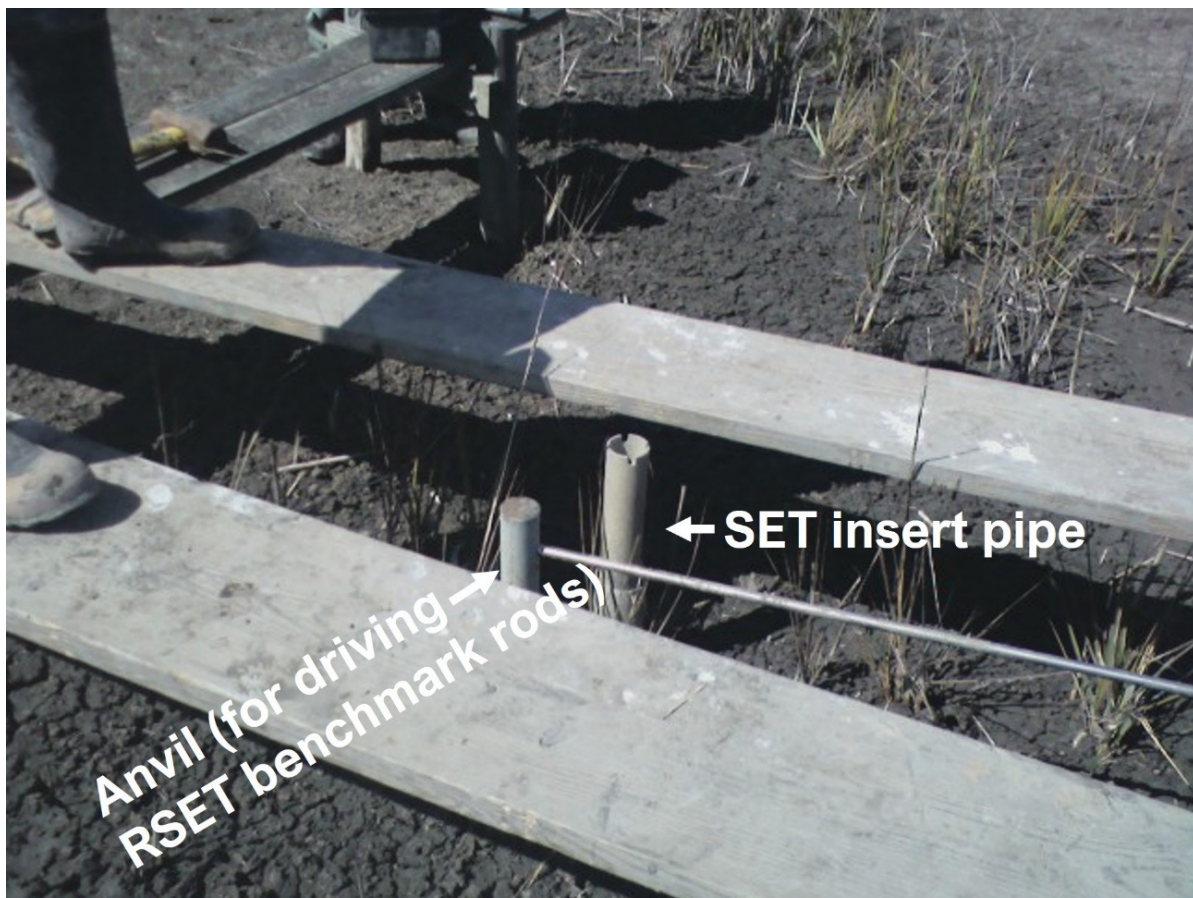
Figure 3. RSET installation adjacent to original SET. Note: gray anvil is on top of the RSET mark rods.
