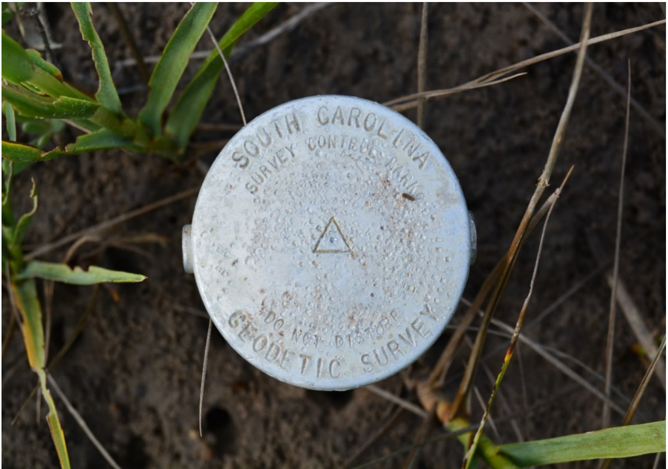
Appendix G, Figure 2. Center point cap used as geodetic control point (center of the triangle) when surveying original SCGS stations.
