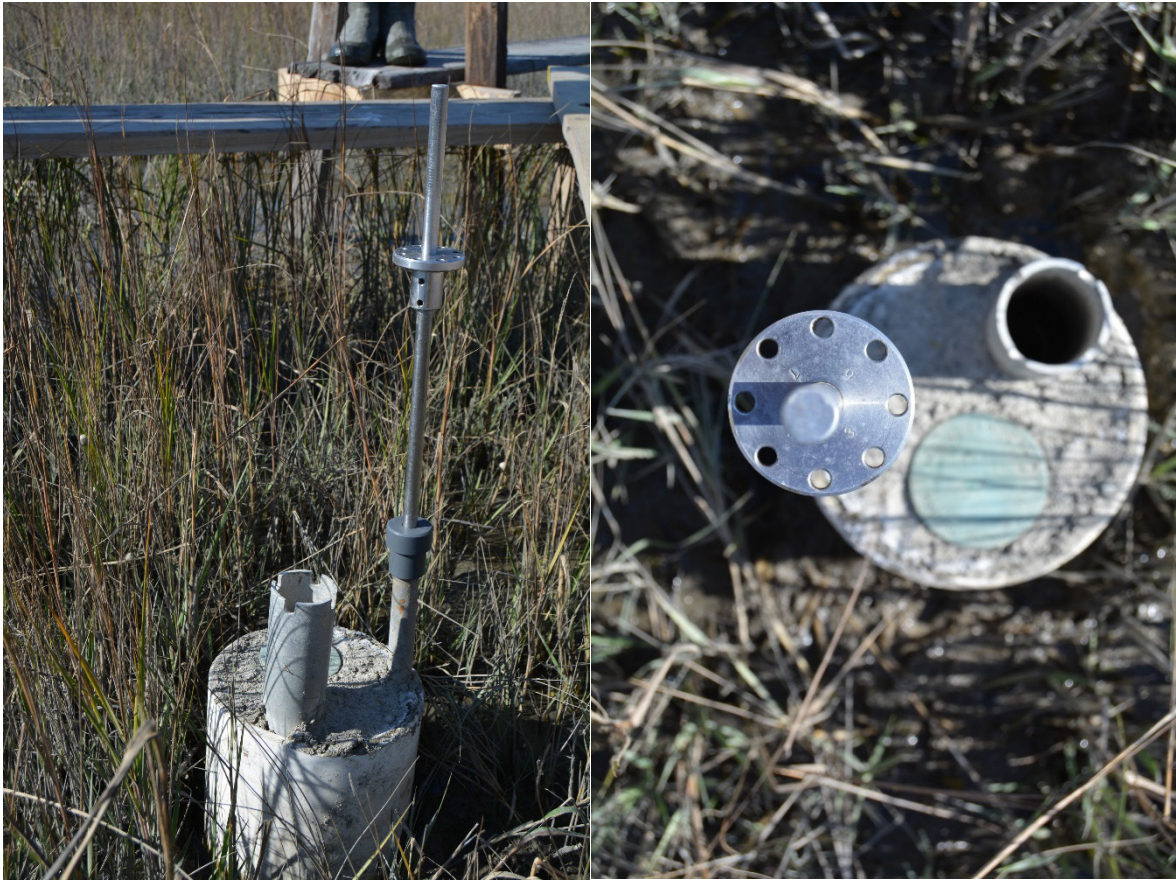
Appendix F, Figure 2. Pictures of the SET insert pipe, the RSET insert collar assembly attached to receiver, and the bronze geodetic control point disk. The left-hand picture shows the locator pin notches in the SET insert pipe (wider pipe on the left). The right-hand picture is an overhead view of the holes in the RSET insert collar assembly. Two pairs of holes are used to measure the four quadrants at each site; they may vary by site. The pairs are oriented at 90-degree angles to one another.
