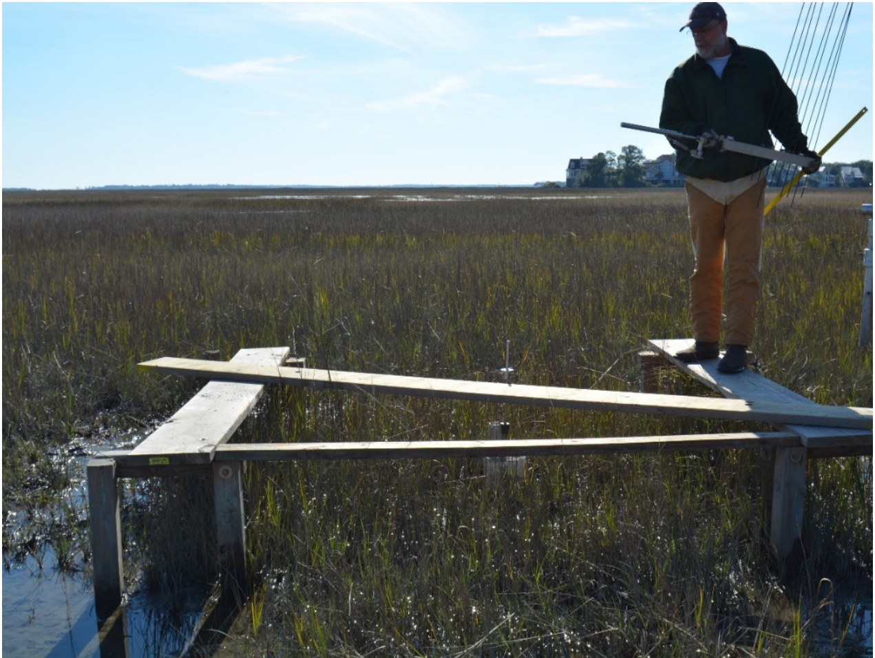
Appendix F, Figure 1. Carrying the RSET instrument to the station with pins inserted. A cross board has been placed across the piers.
