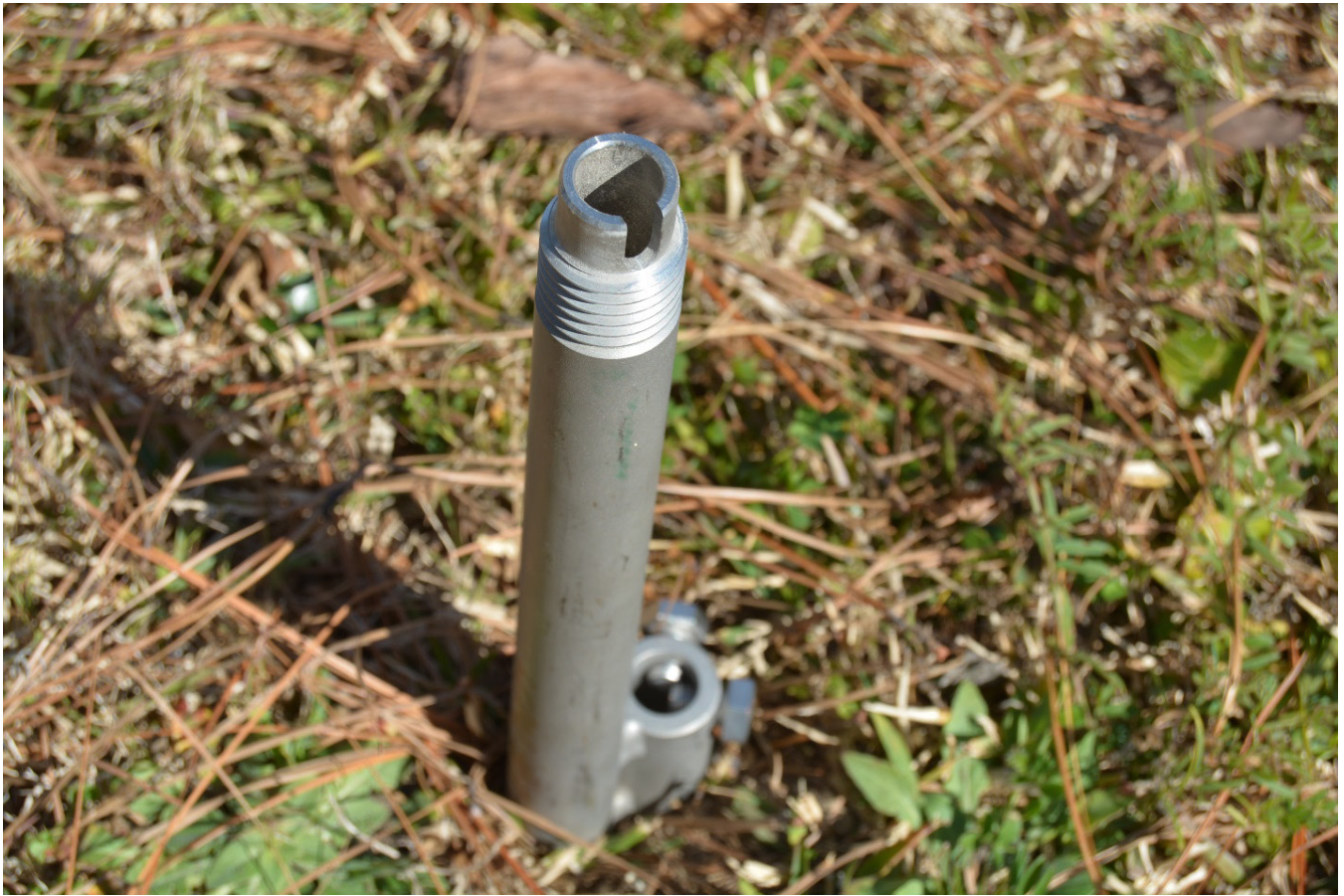
Appendix G, Figure 4. RSET receiver, showing interior cavity where the tip of 2-m carbonite rod is placed (geometry detailed in Appendix H).
