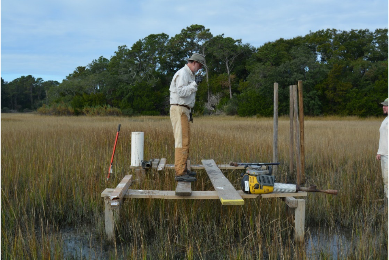
Appendix D, Figure 6. Position two boards across the measuring plot to facilitate locating the middle of the plot and installing the benchmark.
