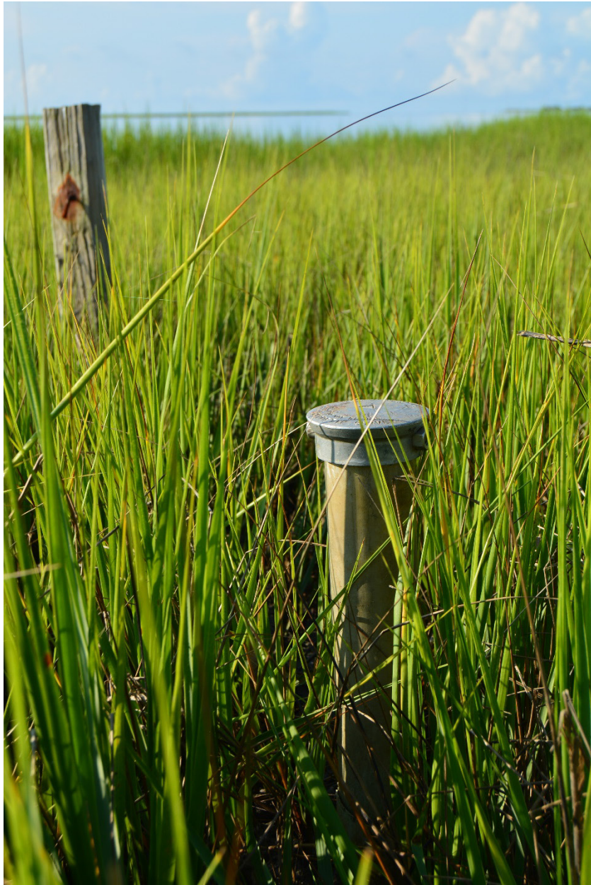
Appendix G, Figure 3. Side view of the SET insert pipe and center point cap.
