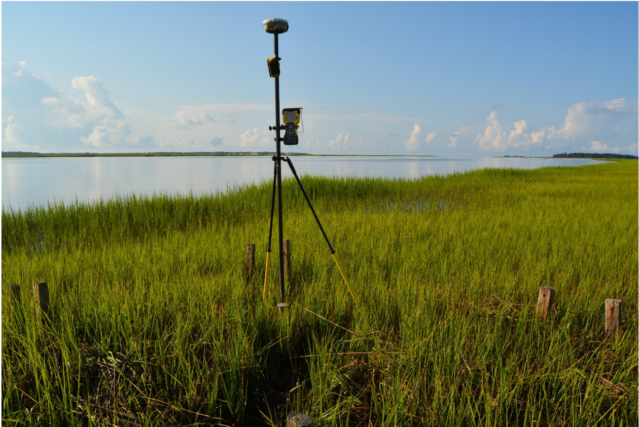
Appendix G, Figure 1. Trimble R8 receiver, TSC2 data collector, wireless MiFi, and bi-pod setup collecting data on a SET station in the field.
