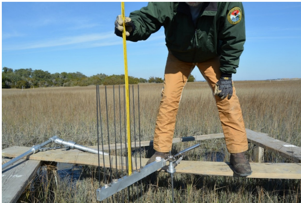
Appendix F, Figure 7. Measuring the length of pin remaining above the table of the RSET instrument. For the RSET, measurements are collected starting at the innermost pin (1) to outermost (9). The instrument may be stamped with these numbers.
