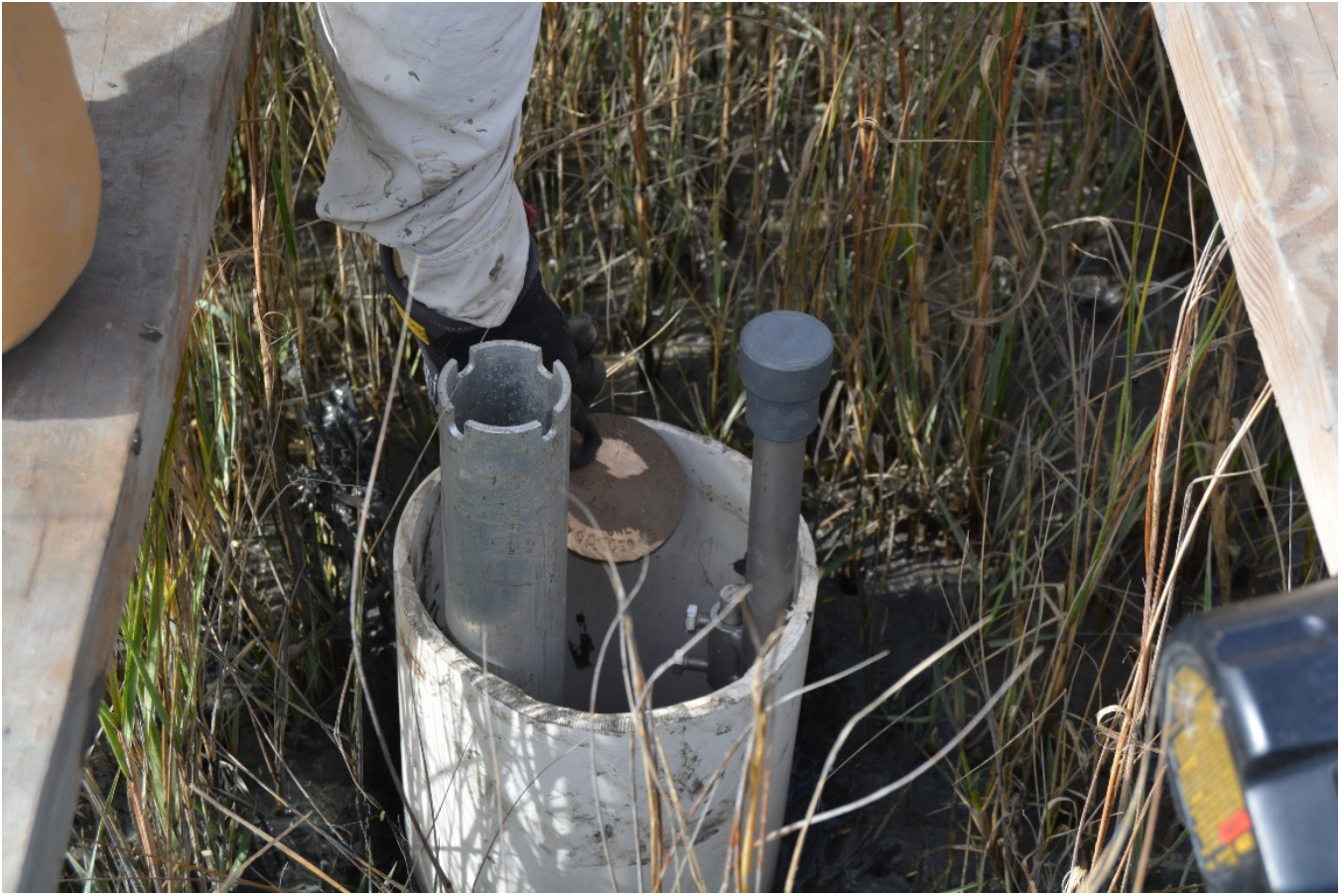
Appendix D, Figure 11. RSET receiver is affixed to steel rod benchmark, and a check is performed to ensure that geodetic disk will fit into PVC collar.
