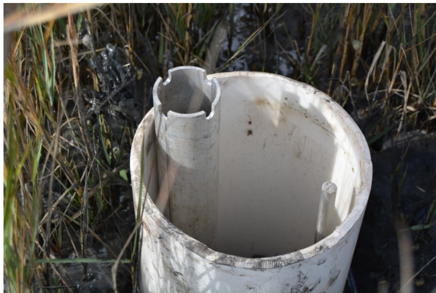
Appendix D, Figure 10. The steel rod is cut below the top of the PVC collar. The insert pipe must remain above the height of the collar.
