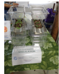
The Tabletop Rainfall Simulator allows SCSU Botany Students to observe the differences in rainfall absorption between the two field samples.
