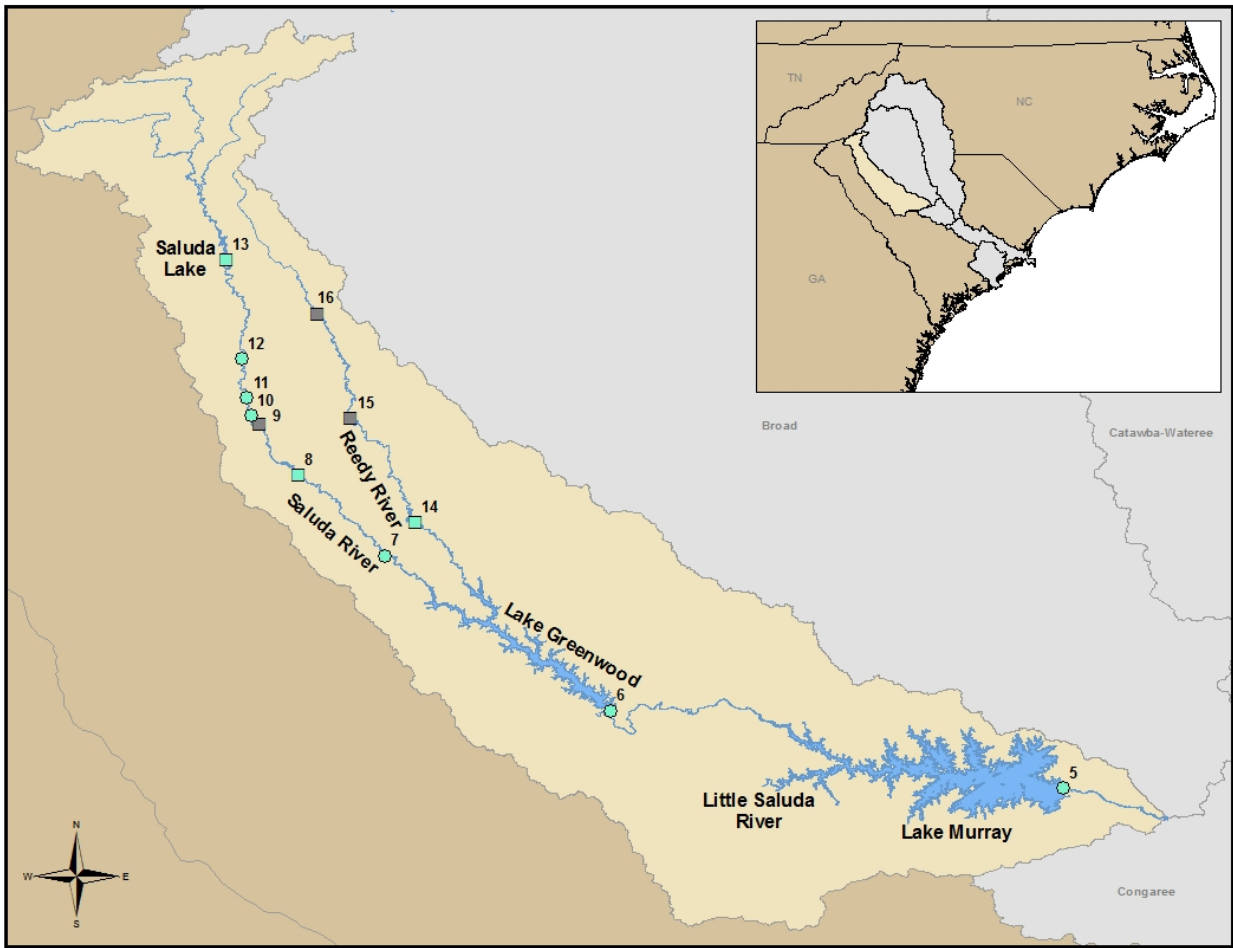
Figure 16. Existing dams in the Saluda River sub-basin. Circles represent facilities that fall under FERC jurisdiction. Squares represent non-FERC facilities (e.g., U.S. Army Corps of Engineers, State, Other). Hydropower facilities are in teal. Numbers refer to dams listed in Table 3.
