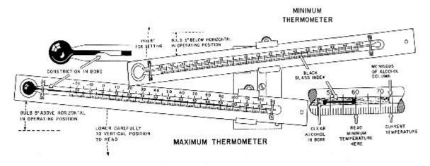
Figure B-1 - Liquid-in-Glass Maximum and Minimum Thermometers
