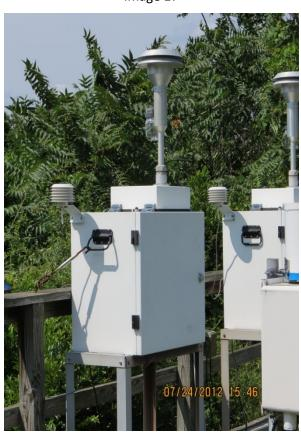
It should be noted that the beehive temperature sensor that is attached to the side of both Thermo Scientific particulate monitors is only five inches away from the top of each unit (Image 17).
