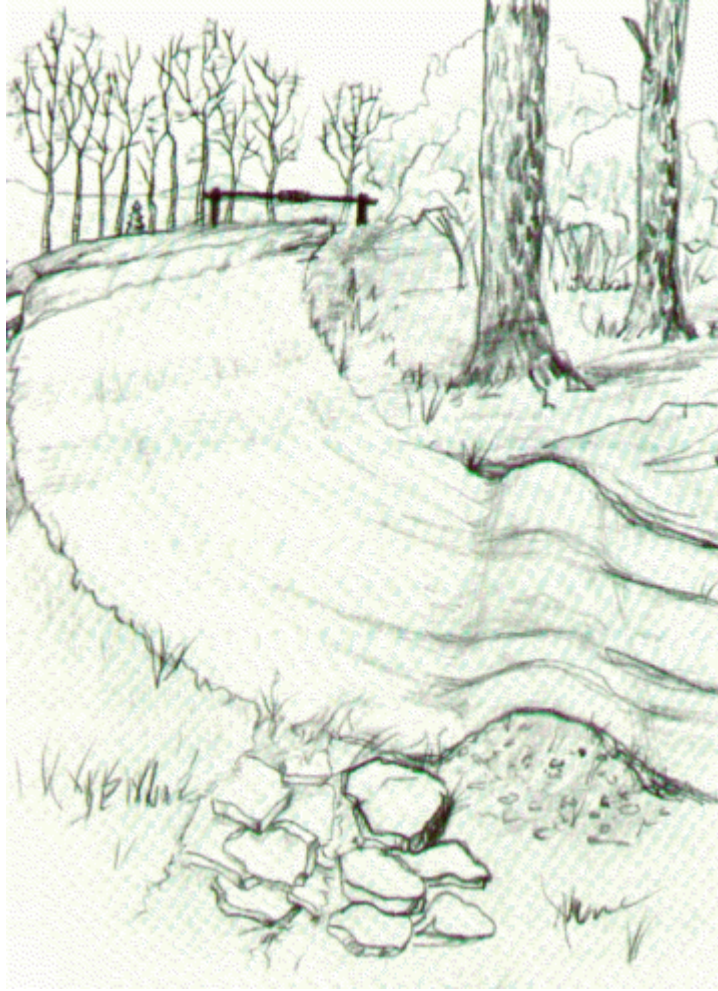
Figure 7. Water bars are used to remove surface runoff when retiring limited use roads.
