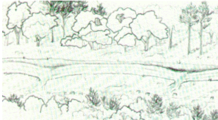
Figure 6. Broad-based dips remove road runoff while allowing vehicles to maintain normal speeds.
