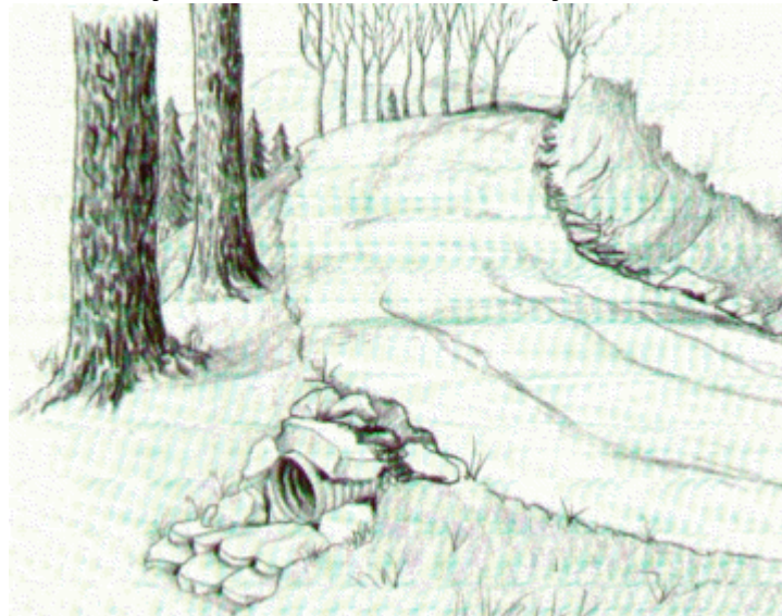
Figure 4. Culverts provide cross drainage for roads with inside ditches.
